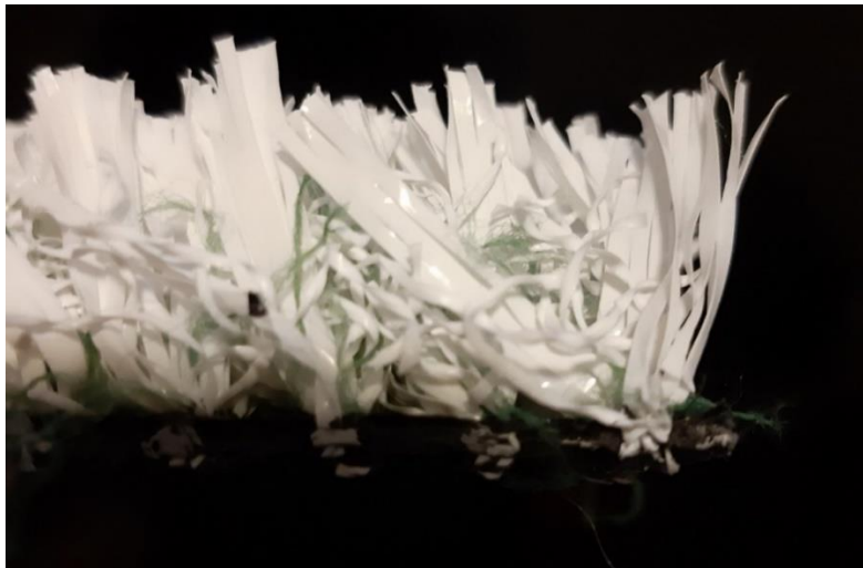
Figure 6: Side profile of a segment of artificial turf. The top of the thicker white yarns is the top layer, and the top of the thinner white yarns is the lower layer.
