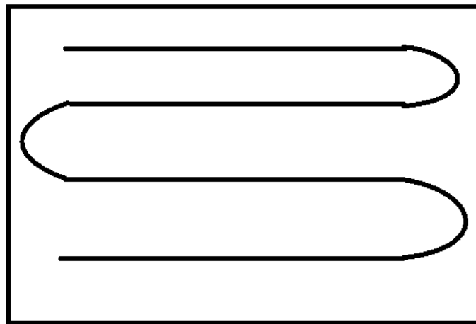
Figure 7: The pattern the swab samplers were brushed across and through the artificial turf.
