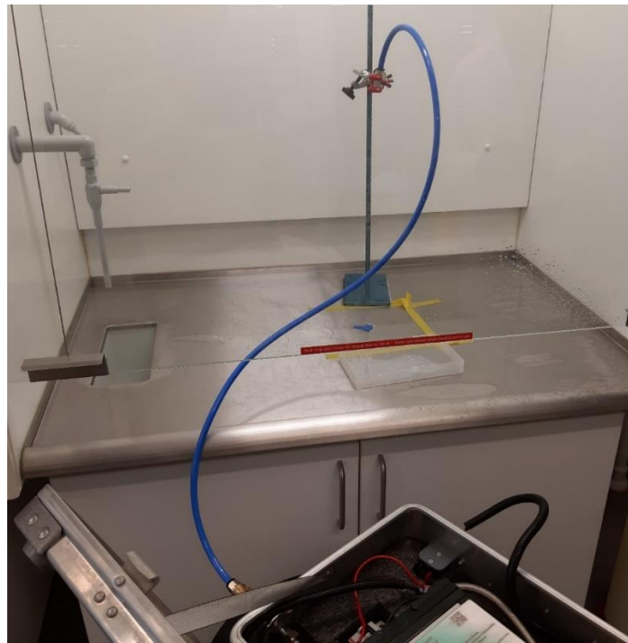
Figure 5: Picture of the experimental setup, the blue tape marks the point below the nozzle and the yellow tape is a 20 cm by 20 cm square around the center which the collection tray is placed in accordance with.
