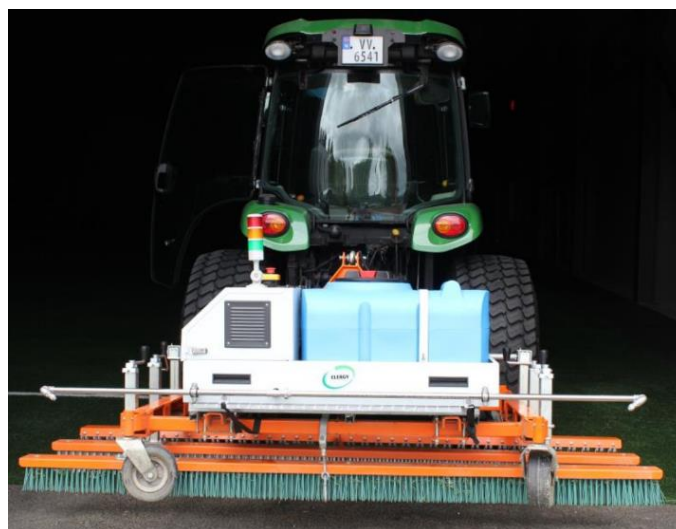
Figure 2: The disinfectant spraying equipment on top of the standard grooming equipment used at Flatåshallen (5).
