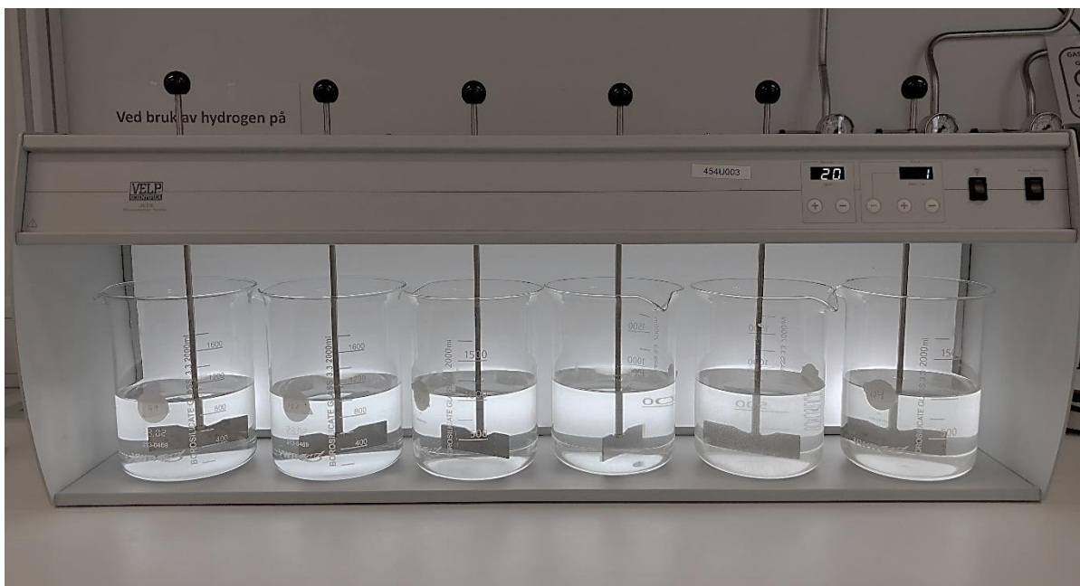
Figure 7: Jar-test set up in multiple stirrer.
