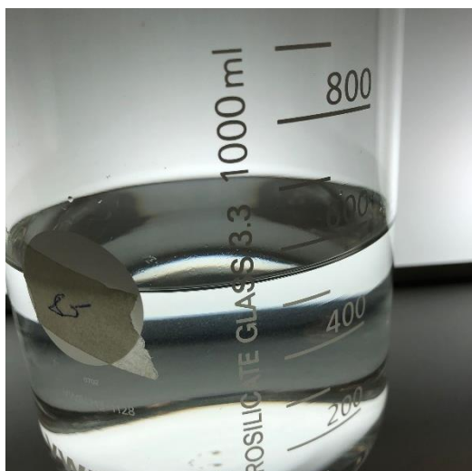
Figure 17: Reaction with Metalsorb ZM 3 and pH = 9.8.
