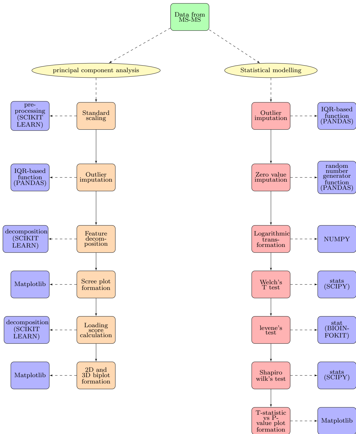
Figure 13: Different components of the data analysis pipeline developed for analyzing the MS-MS data. The original dataset (green) passes separately through two processes (yellow): PCA and statistical modeling. Both processes have different steps arranged in order from top to bottom and connected by solid downward arrows. Steps in principle components are shown in the orange blocks, while steps in the statistical modeling are in the red blocks. The blue blocks connected to corresponding steps by dashed arrows indicate the Python function and the package used (in parentheses) to execute the step. The flow chart was created using LaTeX.
