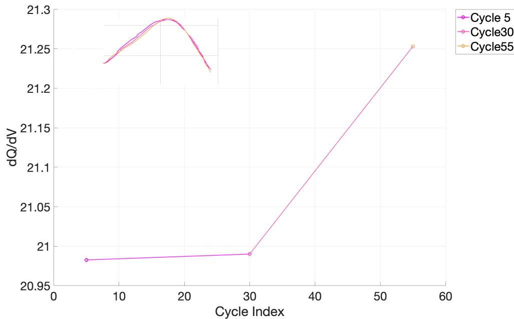
Figure 4.30: Development of the maximum dQ/dV values for Grepow, 45\text{ }^{\circ}\text{C}
