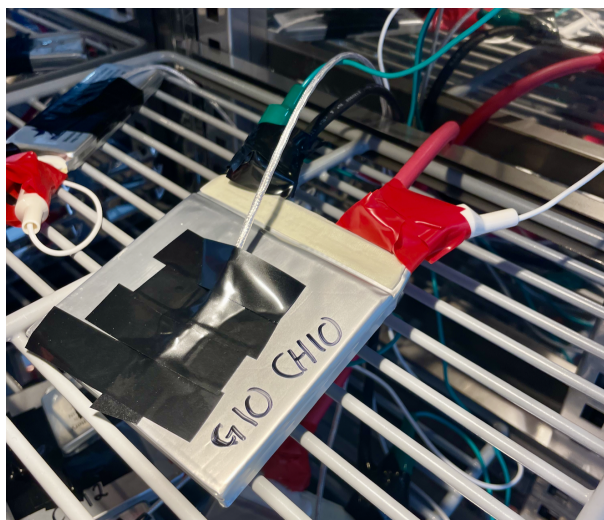
Figure 3.2: How the batteries are connected with cables to the chamber
