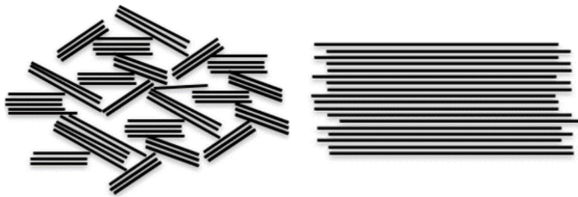
Figure 2.5: The structure of both hard carbon (left) and graphite (right) [56]
