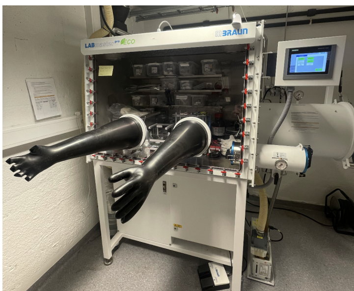
Figure 3.8: The LABmaster pro ECO glovebox utilized for visual inspection
