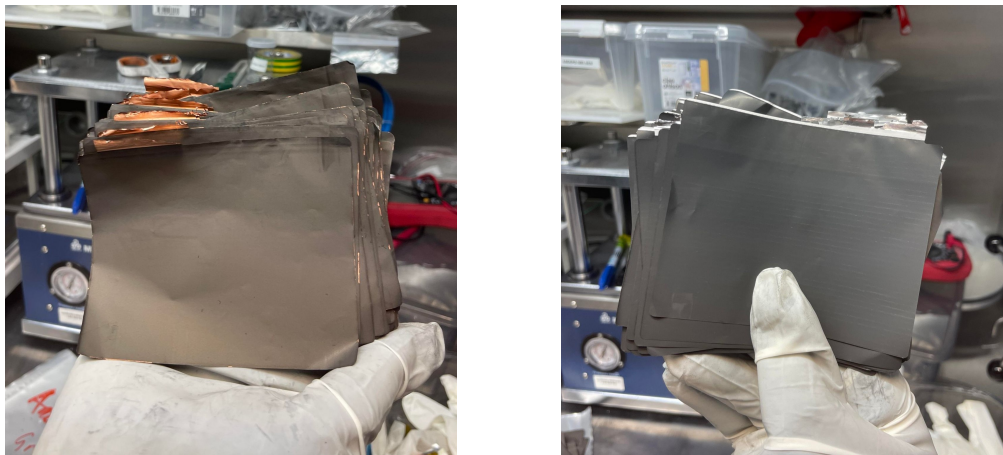
Figure 4.33: The anode layers (left) and cathode layers (right) for a Grepow cell
