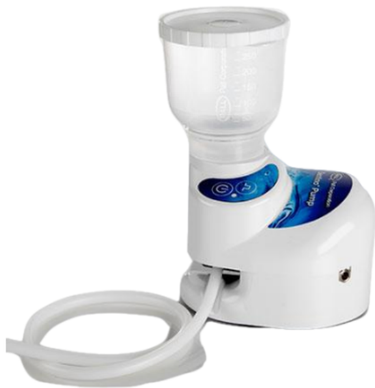
Figur 2: Filterpumpe (Sentino ® microbiology pump, Cytiva ™ ) (24).
