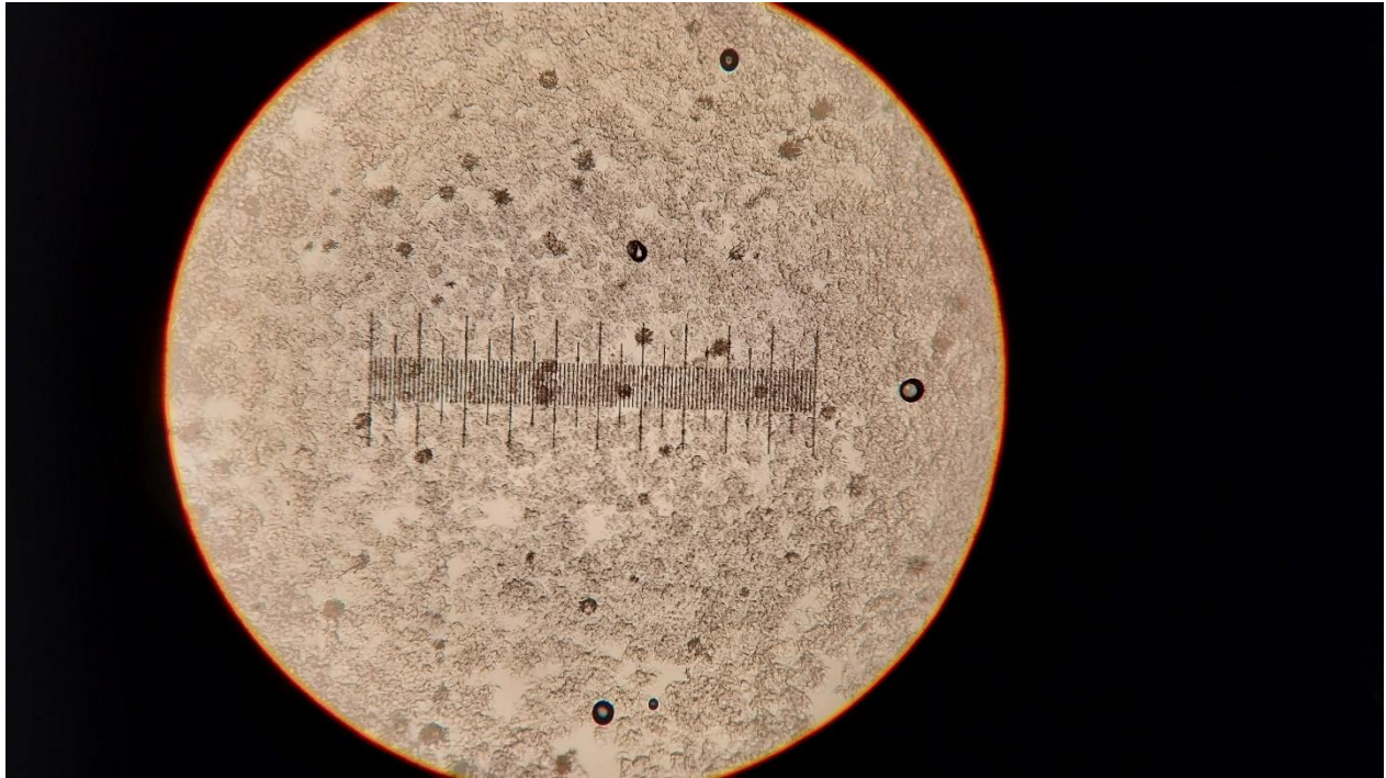
Appendix 10 – An image taken through a Carl Zeiss compound microscope with 4x zoom showcasing the crystalline structures formed during static winterization, while tempering at 4°C.
