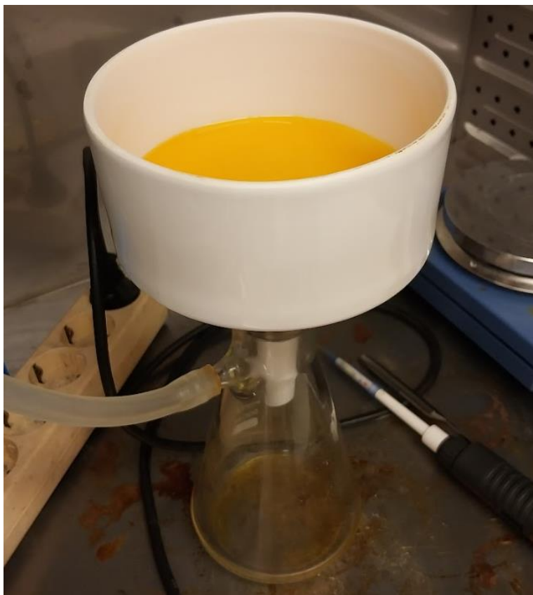
Figure 16: A picture depicting the setup of the Büchner flask, the filter and the tube connecting to the vacuum pump. Notice the presence of the slurry in the Büchner filter and the liquid phase amassing in the bottom of the flask.
