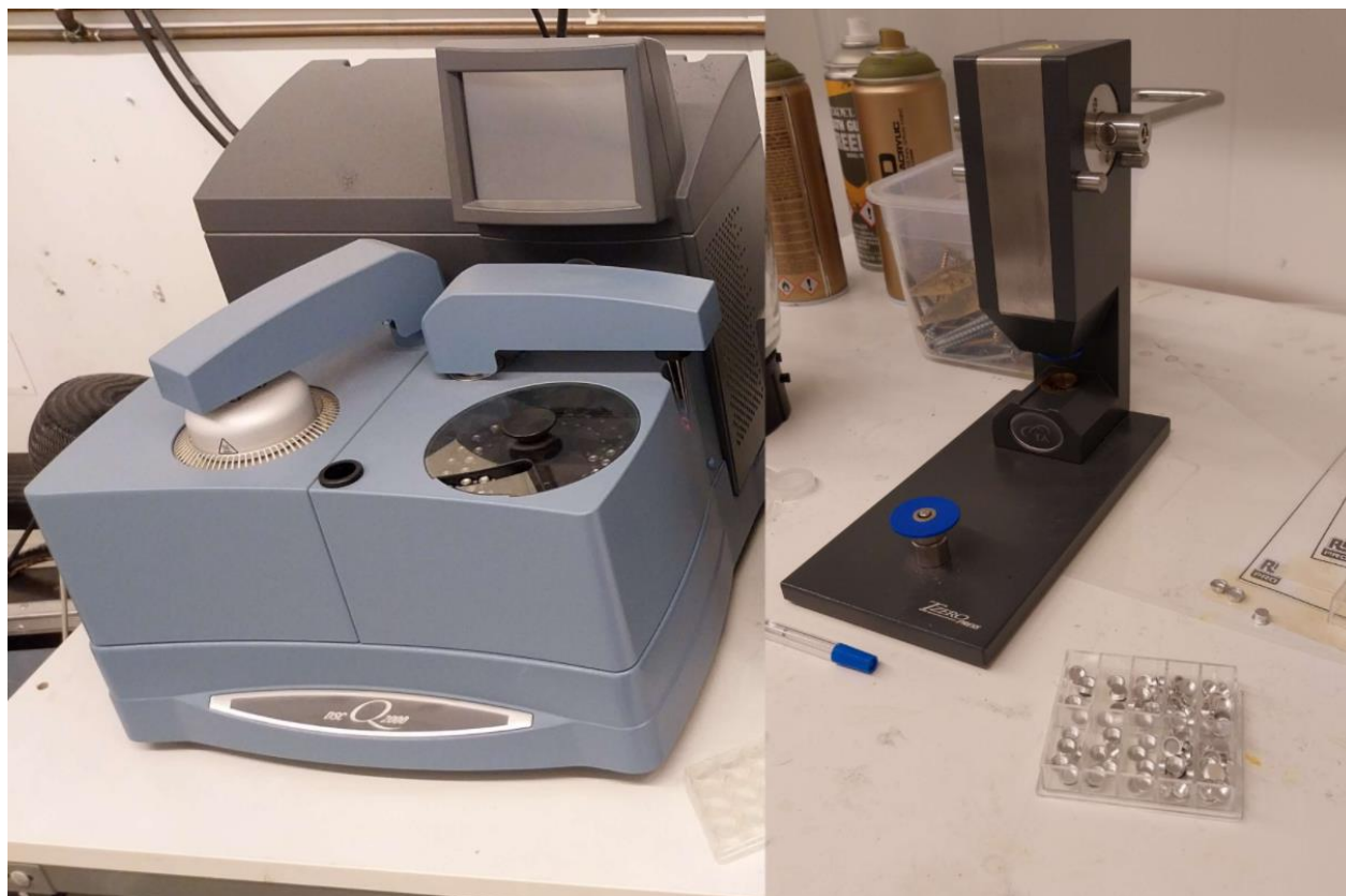
Figure 21: A picture depicting the Q2000 DSC instrument, TZero aluminum pans, and the TZero DSC Sample Encapsulation press used to secure the pans with the sample inside.
