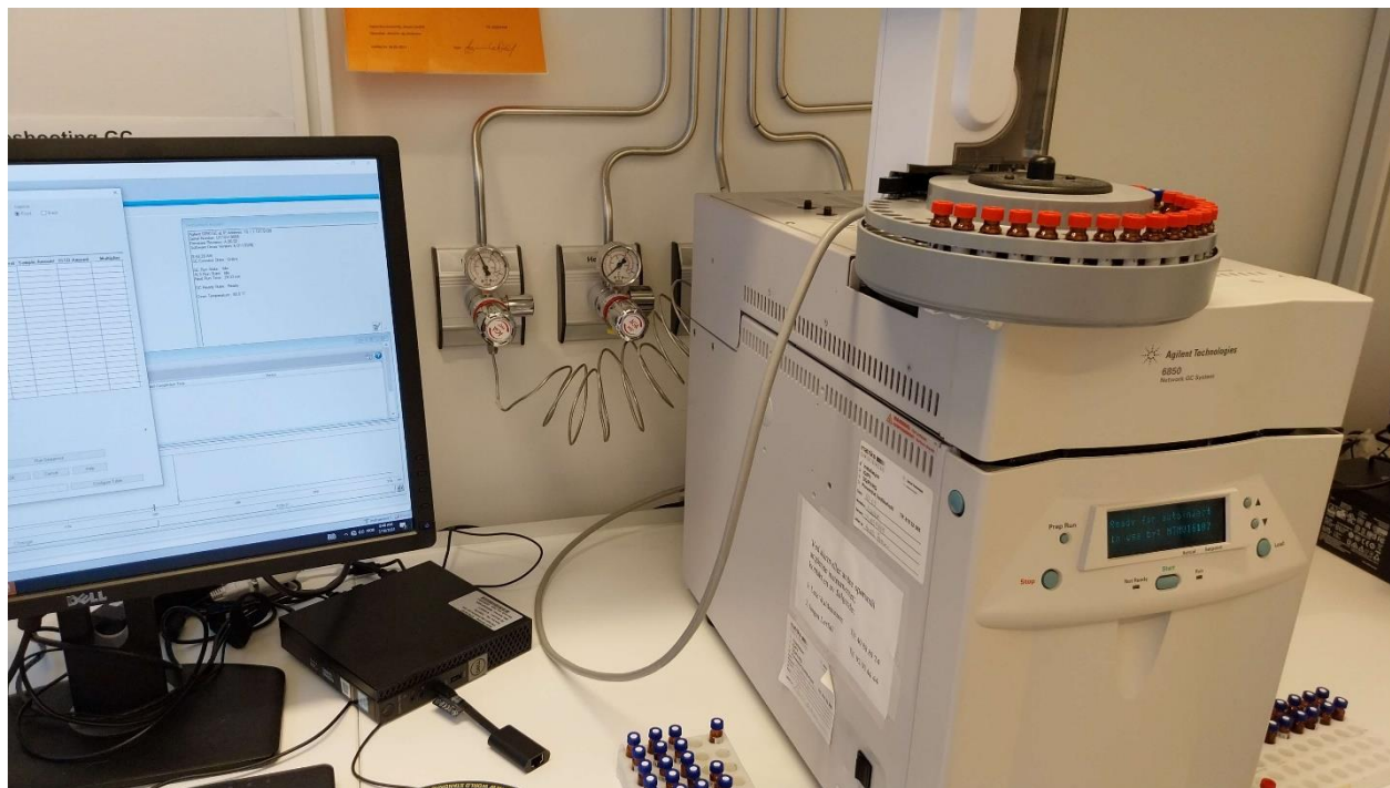
Figure 20: A picture depicting the GC instrument used for analysis of the FAME samples. The depicted GC instrument is an Agilent Technologies 6850 GC networking system.
