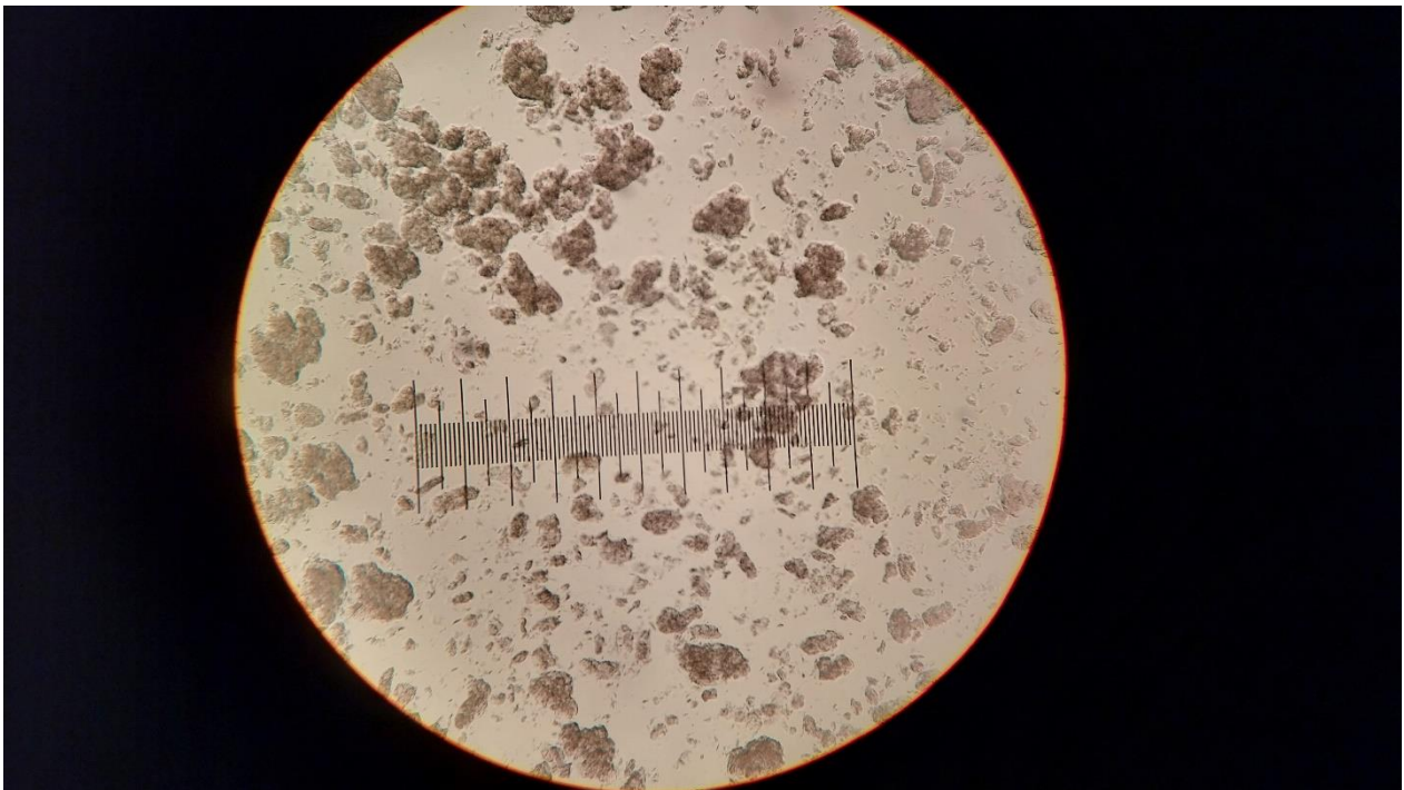
Appendix 4 - An image taken through a Carl Zeiss compound microscope with 4x zoom showcasing the crystalline structures formed during dynamic winterization, while tempering at 12°C.
