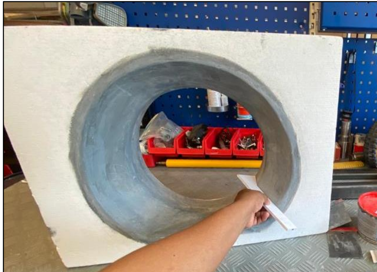
Figure 4-6: Comparing Edge Geometry to Edge Mold for 20° Linear Inlet.
