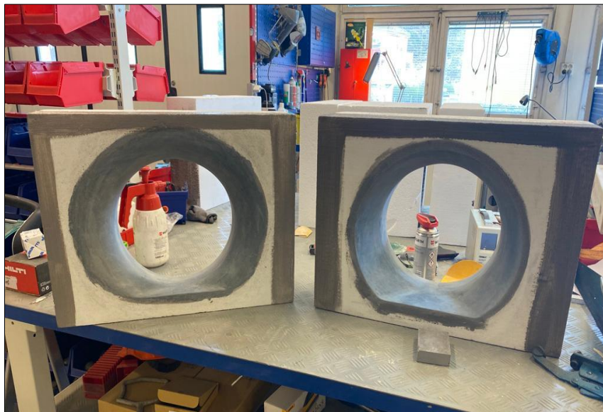
Figure 4-5: Sample of Finalized Linear and Non-Linear Inlets with Bevel Angle 20^\circ .
