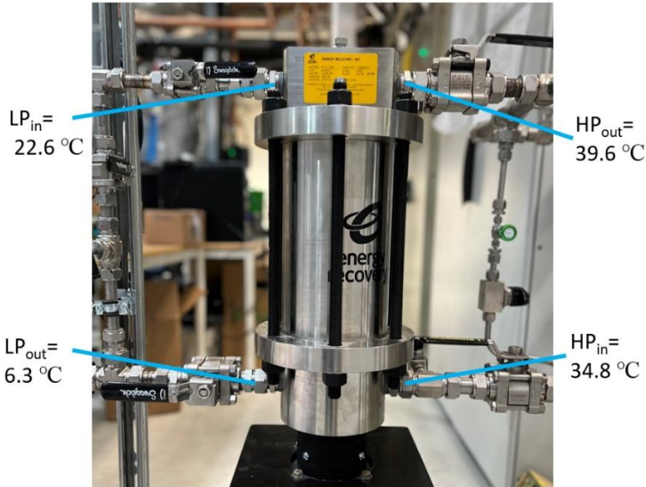
Figure 4.7: Experimental PX ports (inside) temperatures of 35 °C case
