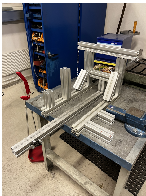
Figure 18: Model of test rig constructed from aluminium frames.
