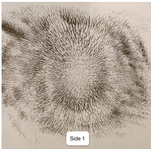
Figure 37: Magnetic field shown with iron filings from the "strong" side of the magnet, side 1.
