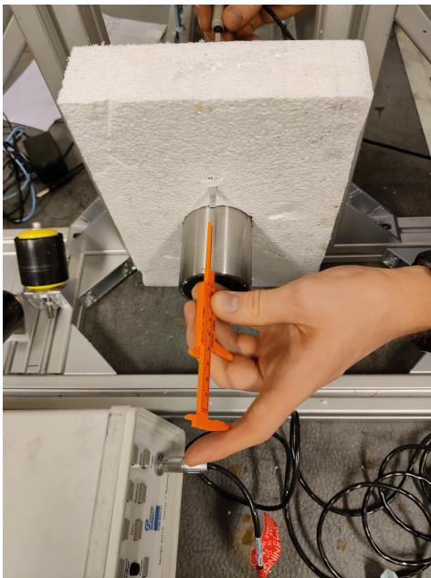
Figure 13: Gaussmeter-probe held in place with Styrofoam. Position controlled with vernier.
