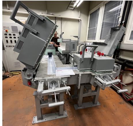
Figure 34: LML with open lids revealing the refractory lane, and the heat elements in the lids.
