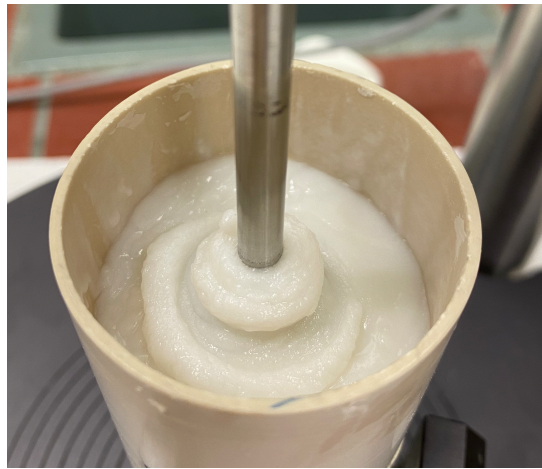
Figure 4.3: Illustration of the Weissenberg effect. The picture is from an experiment conducted on Exilva with a concentration of 3.60% with a V40/20 vane. It is clearly seen that the material is drawn upwards around the vane shaft, resulting in an alternated resistance to flow.
