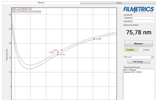
(a) Reflectometer measurements of the film grown for one minute
