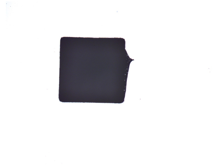
(b) Aperture after exposure and lift-off with dose 250 \mu\text{C}/\text{cm}^2
