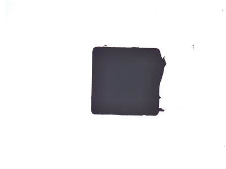
(d) Aperture after exposure and lift-off with dose 300 \mu\text{C}/\text{cm}^2
