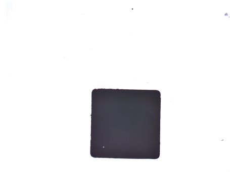
(f) Aperture after exposure and lift-off with dose 350 \mu\text{C}/\text{cm}^2
