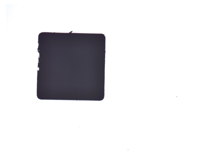
(h) Aperture after exposure and lift-off with dose 400 \mu\text{C}/\text{cm}^2
