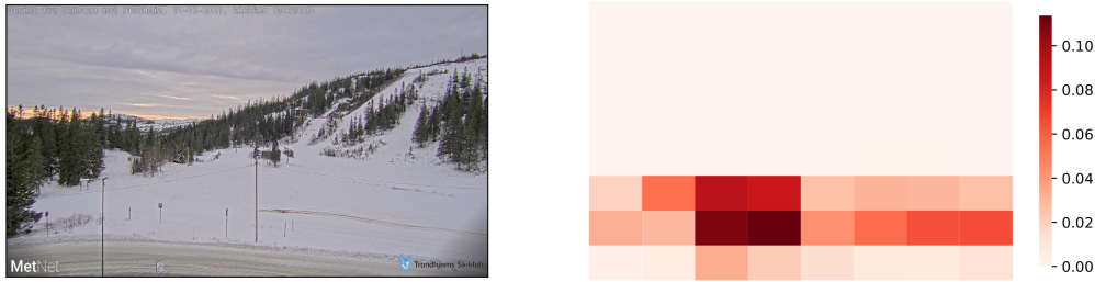
Figure 3: Visual attention model, as calculated by the device manager module over the entire range of images used as a test set. Darker cells are the image regions in which more often persons have appeared.
