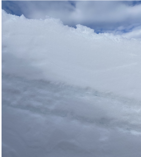
Figure A.1.1: An example of snow stratigraphy, showing two distinct ice layers close to the snowpack’s surface. The picture is taken during this study.
