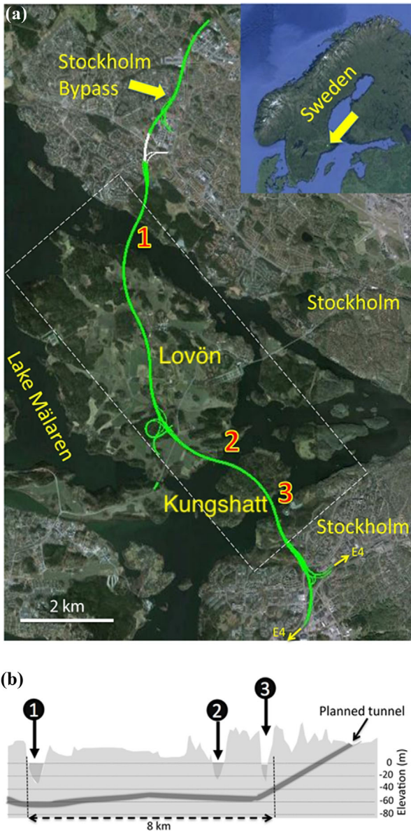
Figure 1 Location of the study area. (a) The Stockholm Bypass (Förbifart) project. The planned bypass is shown with the green track. (b) Profile section of water passages, marked by numbers 1 to 3, showing the location and depths to the top of the tunnel. The inset map in (a) shows the location of the study area in Sweden.
