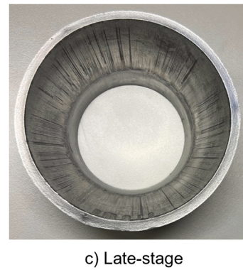
Fig. 10. Fracture initiation on the sample surfaces.
