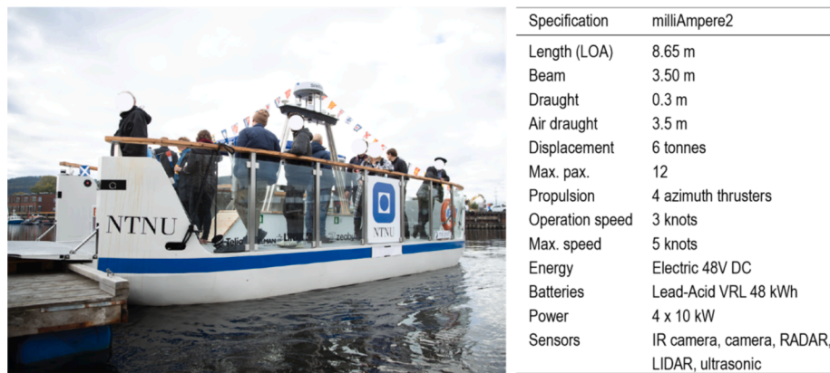
Fig. 2. The milliAmpere2 and some of its main specification. (Photo: Kai T. Dragland, NTNU).
