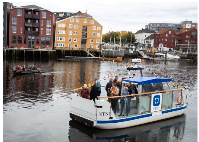
Fig. 1. The autonomous urban passenger ferry milliAmpere2 during its trial operation in September and October 2022 in Kanalen, Trondheim, Norway. The traditional ferry service “Ferry Man” is to the left. (Photo: Kai T. Dragland, NTNU).
