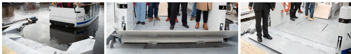
Fig. 6. The special dock at Fosenkaia (left) and how the latch worked (middle and right). (Photo: Kai T. Dragland, NTNU).
