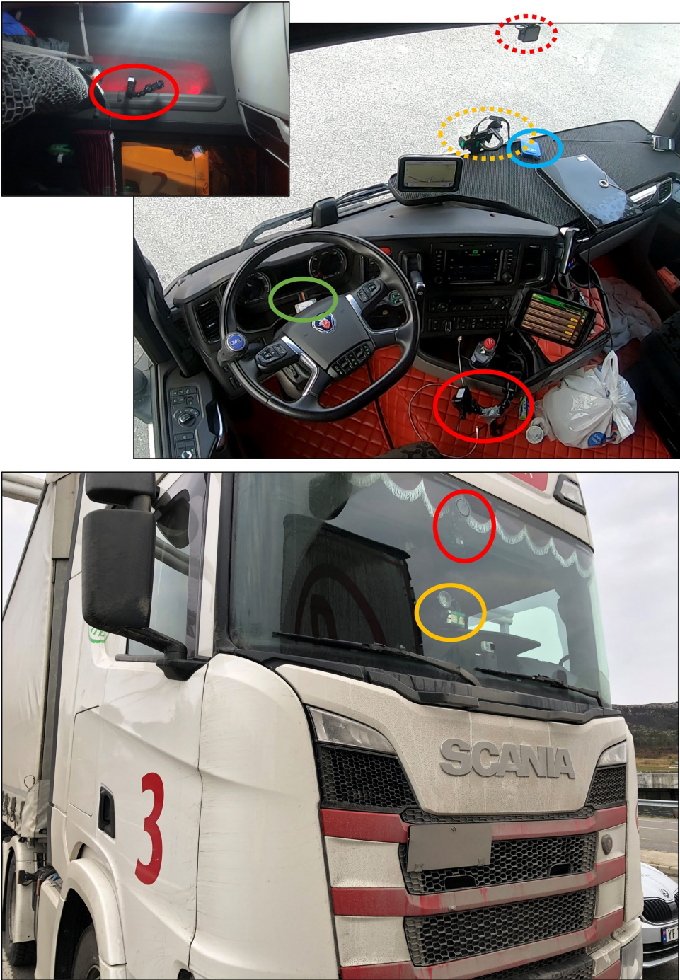
Figure 12: Instrumentation: GoPro (red), SQ11 (green), radar (yellow) and VBOX (blue).
