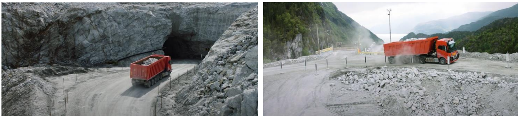
Figure 2: Automated haulage of limestone at Brønnøy Kalk [35]. Left: Tunnel entry after sharp left-curve. Right: Crusher site
