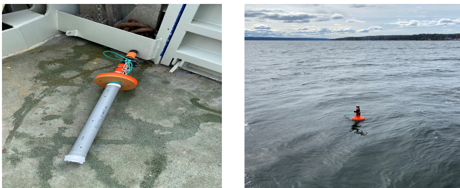
Figure 1.2: Photos of experimental drifters used for drift trajectory monitoring during a cruise in Inner Oslofjord on the 27.04.2023. Drifters can be used to gather current observations in a specific area of interest.
