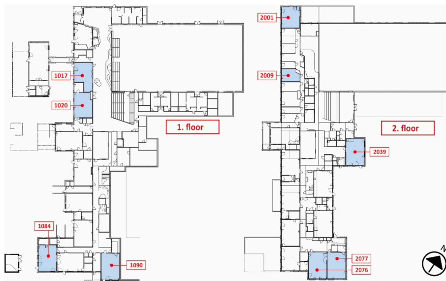
Fig. 5. Floor plan for 1st floor (left) and 2nd floor (right) of Ydalir School with the representative rooms highlighted in blue. Measurement data is logged in the representative rooms only. (For interpretation of the references to colour in this figure legend, the reader is referred to the web version of this article.)
