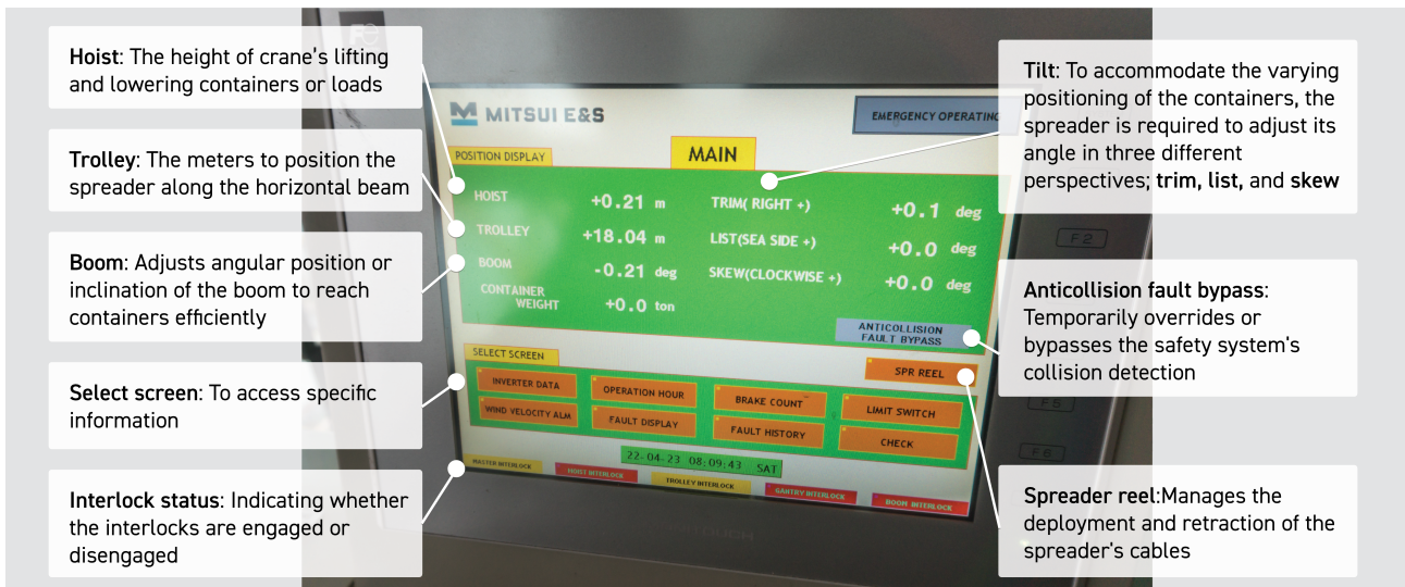
Figure 2: An example of how we inspected every UI element that exists in the GUI used for operating STS cranes.
