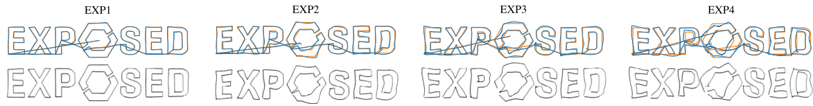
Fig. 9. Comparison between reference and measured trajectories. The top row shows the reference trajectory (orange) along with the trajectory measured by the motion capture system (blue). The bottom row displays contrast adjusted photographs of the resulting drawings.
