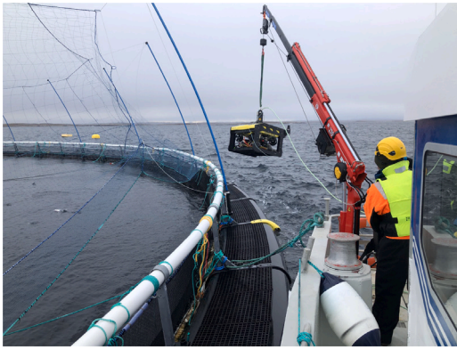
Fig. 1. Exemplary image of manual ROV launch and recovery operation.
