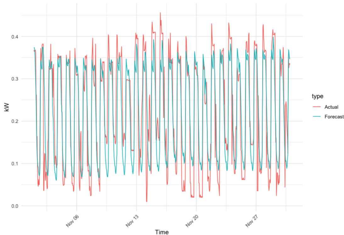
Figure 5.3.9: The actual hourly consumption vs the forecasted demand from the ARIMA model II in 5.3.3 for medical light consumption Chiwoza November 2023.
