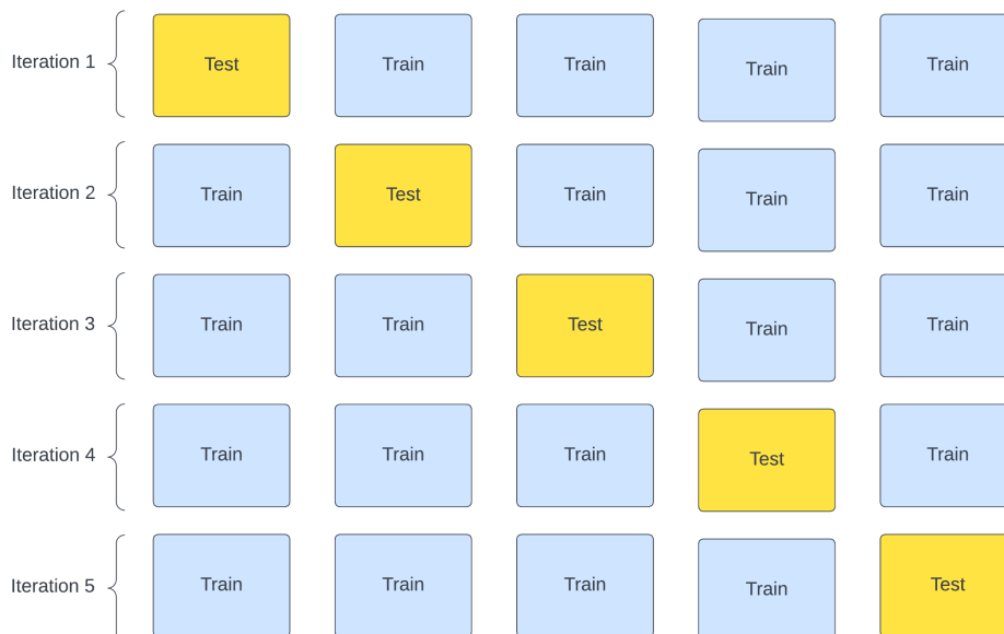
Figure 3: Illustration of K-fold Cross-Validation Process with Five Iterations - Author's own illustration - Adapted (Müller and Guido, 2016, p.252)
