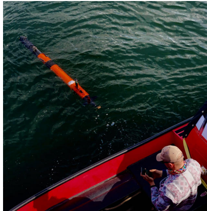
Figure 2.5: LAUV-Thor undergoes remote operation check before its expedition.
