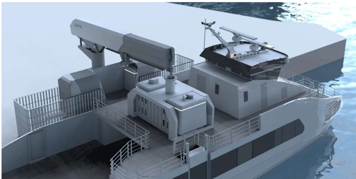
Figure 2-10: Norled Battery-Hybrid Ferry with SHIFTR autonomous battery change robot. Image Credit: Norled [53]
