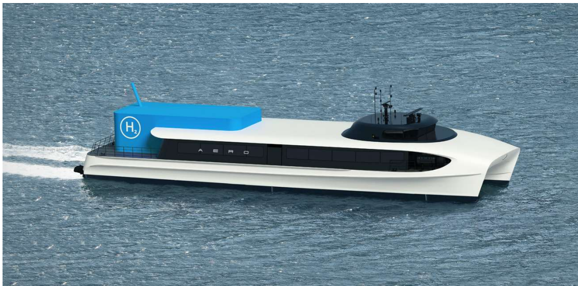
Figure 2-9: Aero. Hydrogen fast ferry concept by "Brødrene Aa" in 2019. Image Credit: Braa.no [20].
