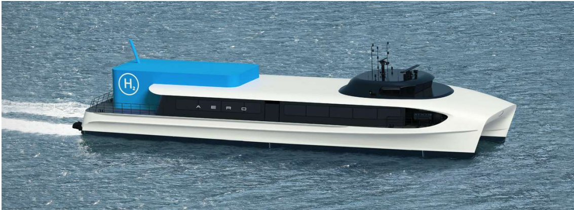
Figure 1-4: Aero. Hydrogen fast ferry concept by "Brødrene Aa" in 2019. Image Credit: Braa.no [20].
