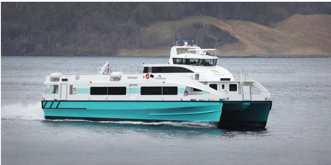
Figure 2-8: MS Terningen. Currently (2023) used diesel-powered vessel with a light-weight carbon fibre hull, by "Brødrene Aa". Image credit: "Braa.no" [49].
