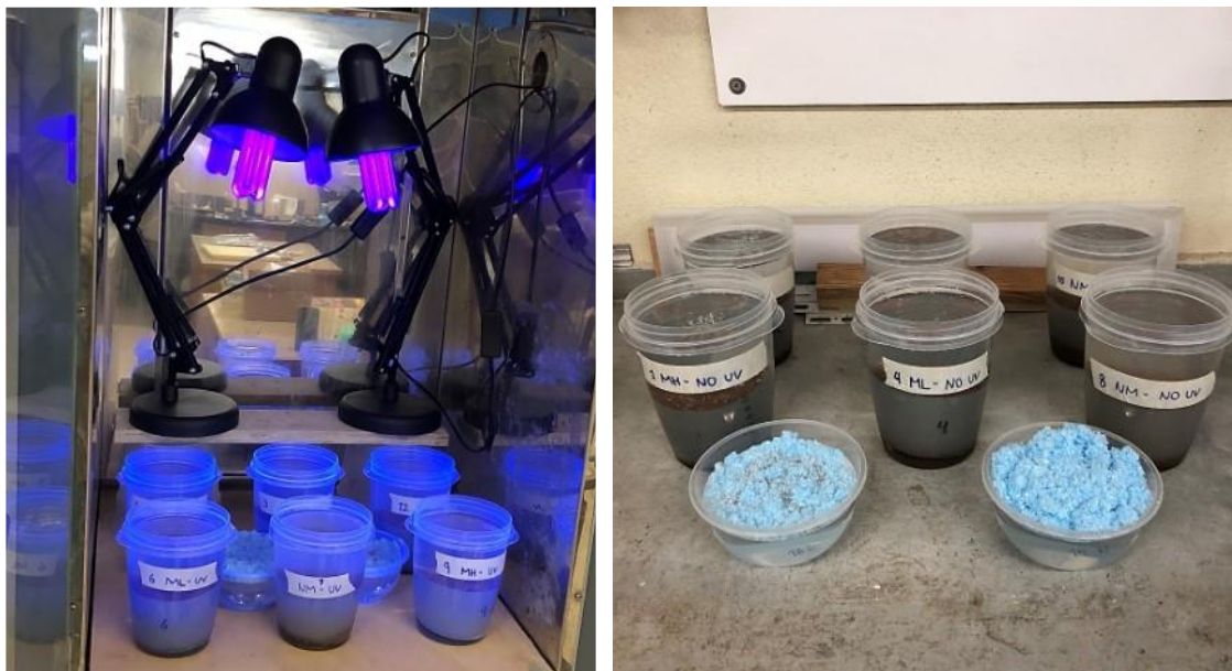
Figure 3.9. Experimental setup of samples suffering UV exposure to the left and no UV exposure to the right.
