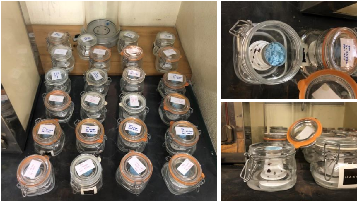
Figure 3.13. Experimental setup of the procedure of the water retention curve. Samples NM, ML and MH were placed in jars with different NaCl solutions. Red labels correspond to samples left to be dried and blue labels corresponds to samples left to be wetted.
