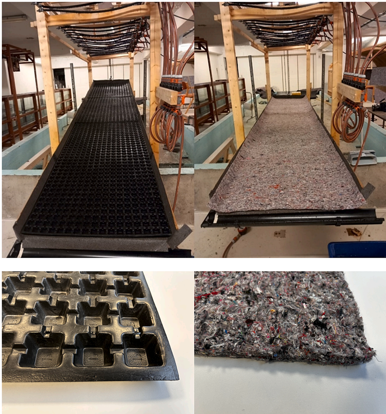
Fig. 1. The test bed used in the study. Left: the hard plastic egg-shape drain mat (ES). Right: the retention mat (RM).
