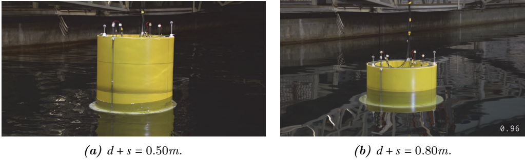
Figure 4.1: Photos of the model during tests in regular waves for both draughts. November 2018.
