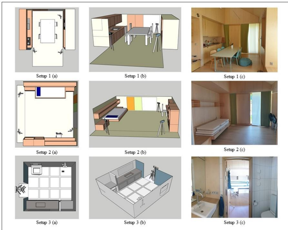
Figure 3-4. From Paper 9: Case scenario and experimental design setups in the smart living lab
