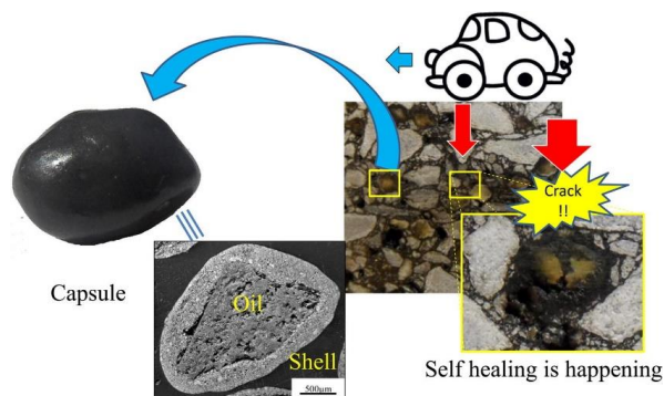
Figure 4 Characterization and healing process of saturated porous aggregates encapsulate rejuvenators [17]
