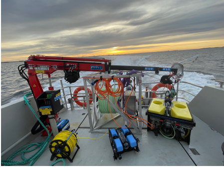
(a) The Argus Mini (yellow) and BlueROV2 (blue) ROVs at the back of the research vessel M/S Torra. Photo: Eleni Kelasidi.
