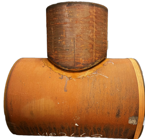
Fig. 1. An example of a large tubular T-joint used in offshore structures, which was used for real-world data collection in this work.
