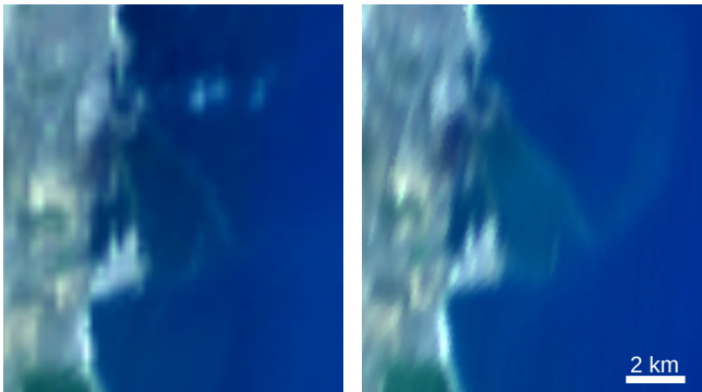
Fig. 3: Nadir pointing (left) and slew (right) RGB images over the port of Constanța, Romania. Zoom-in on the images in Figure 2, bilinearly resampled to the same scale with contrast enhanced.
