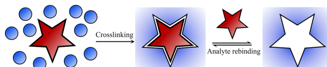
Fig. 1. Simple diagram of the molecular imprinting principle. Crosslinking of polymer surrounding an analyte result in a cavity with affinity for that analyte.
