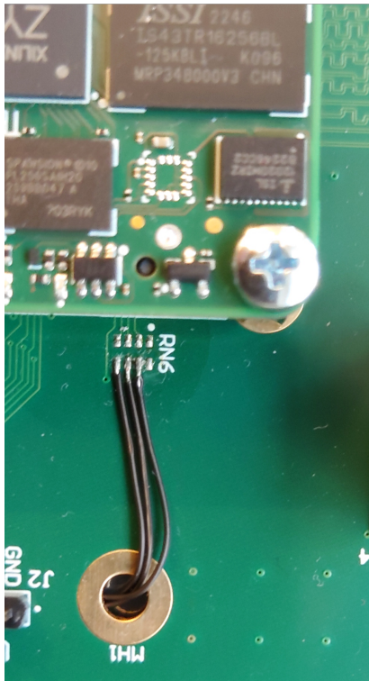
(a) Photo showing the removal of resistor bank RN6 and wires soldered to SPI pins.
