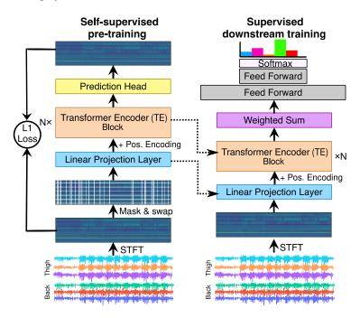
Fig. 1: Illustration of the SelfPAB method, consisting of two parts, the self-supervised pre-training (left) and the supervised downstream training (right).
