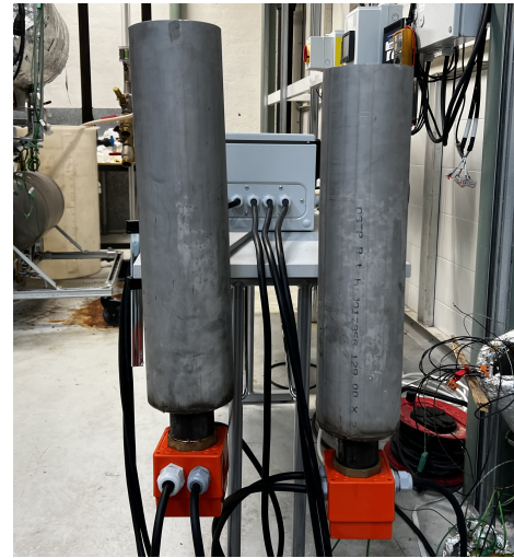
(b) The heating element installation in metal cylinders.
