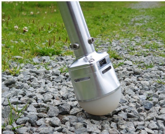
Fig. 1: The developed TRACEPaw system delivering contact force estimation and terrain classification on the edge for legged robots.
