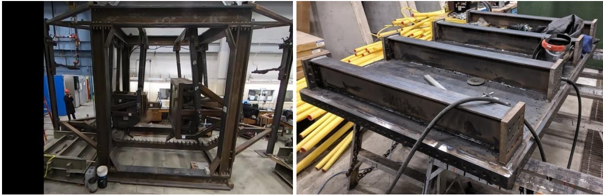
Figure 8: Large double-pendulum apparatus (left) and replaceable stiffened hull panel (right).
