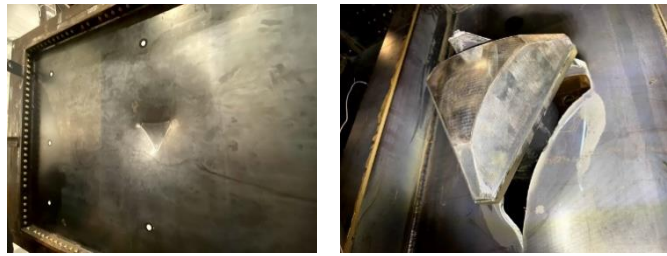
Figure 11: Plating after 1st non-smooth impact (left) and after 2nd non-smooth impact (right)
