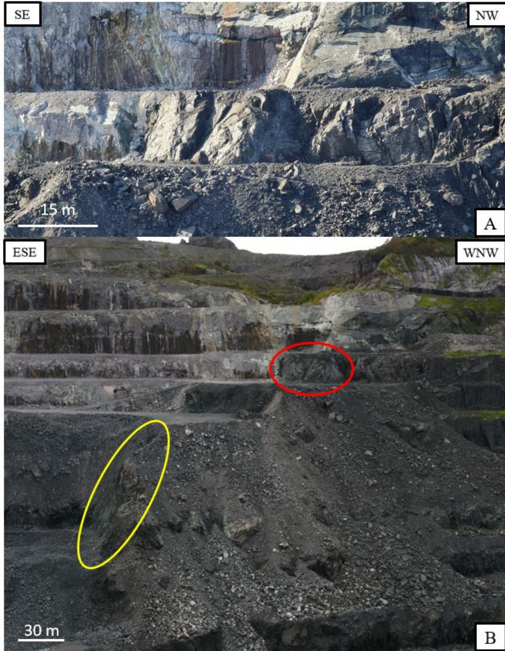
Figure 20: Appearance of alteration zone 155-1. (A) The Stabben alteration zone (155-2) is a large, 40-50 m wide, zone of altered rock. (B) An area with similar green colour (within yellow circle) as the Stabben alteration zone (within red circle) is located further down in the pit, but was not investigated due to accessibility. Bench for scale.
