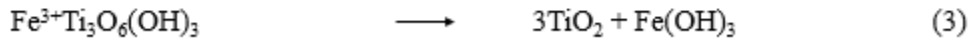
Figure 9: The continuous reaction series established by Mücke & Bhadra Chaudhuri (1991) where ilmenite alters to rutile or leucoxene through pseudorutile. (1) Alteration of ilmenite to pseudorutile by oxidation and leaching. (2) Alteration of pseudorutile to leucoxene by leaching and hydrolysis. (3) Alteration of leucoxene to rutile by disintegration and dehydration.
