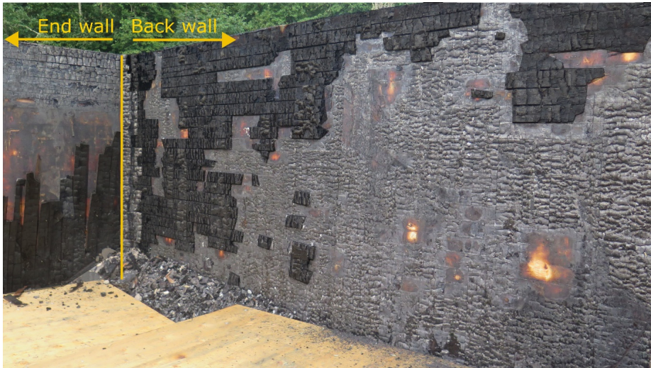
Fig. 42 Charring of the back wall close to the left end wall of #FRIC-02. The back wall is less charred closer to the end wall. The bright spots are fresh wood and show areas that recently have been exposed due to the fall-off of the layer above. A black colour filter has been added to the image to separate the remaining layers better.
