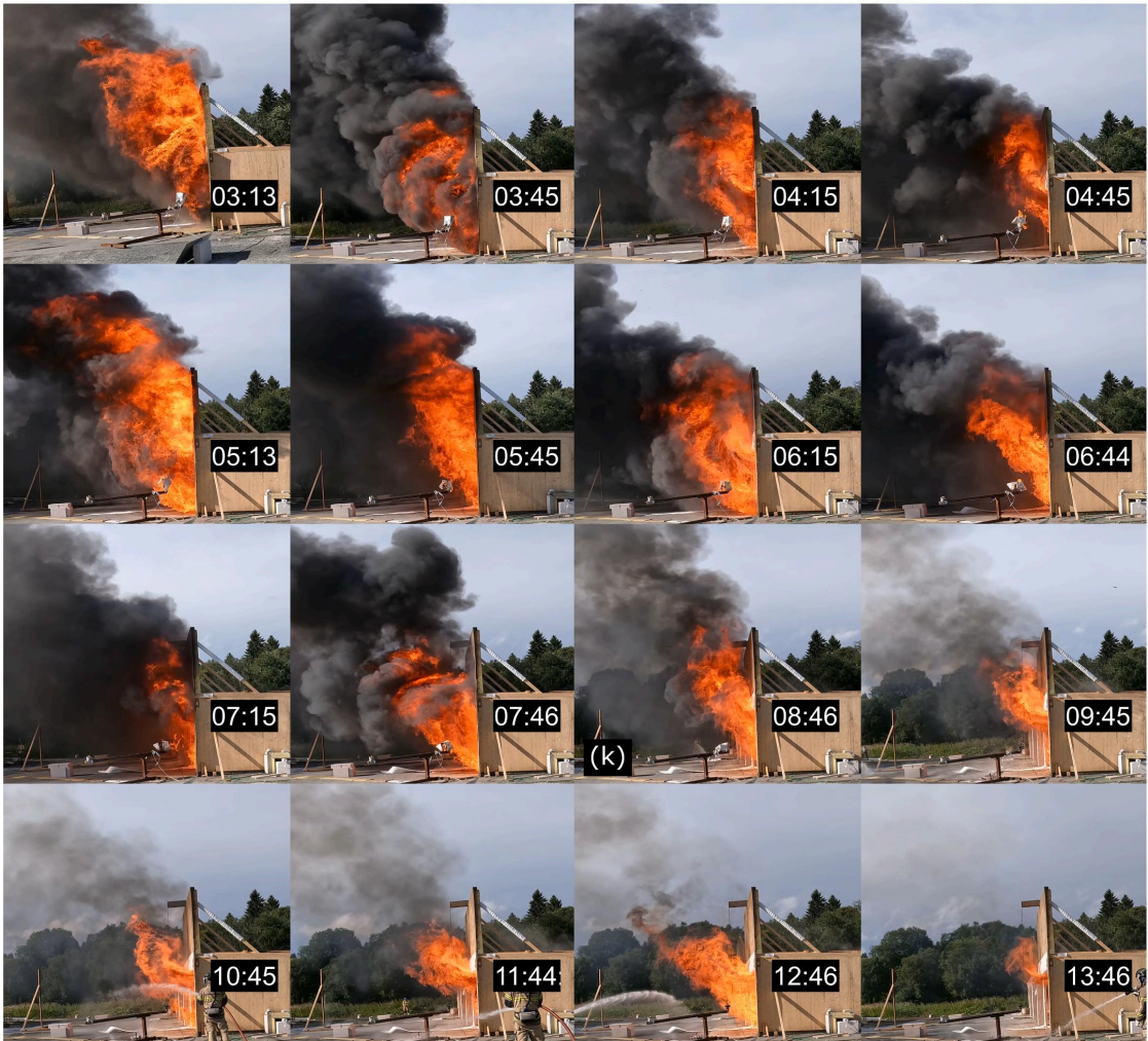
Fig. 18. Side view of external flame emerging from Window 4. Time (mm:ss) after ignition. The given times might deviate slightly ( \pm 1 s) from the exact times as the start of ignition was not recorded.
