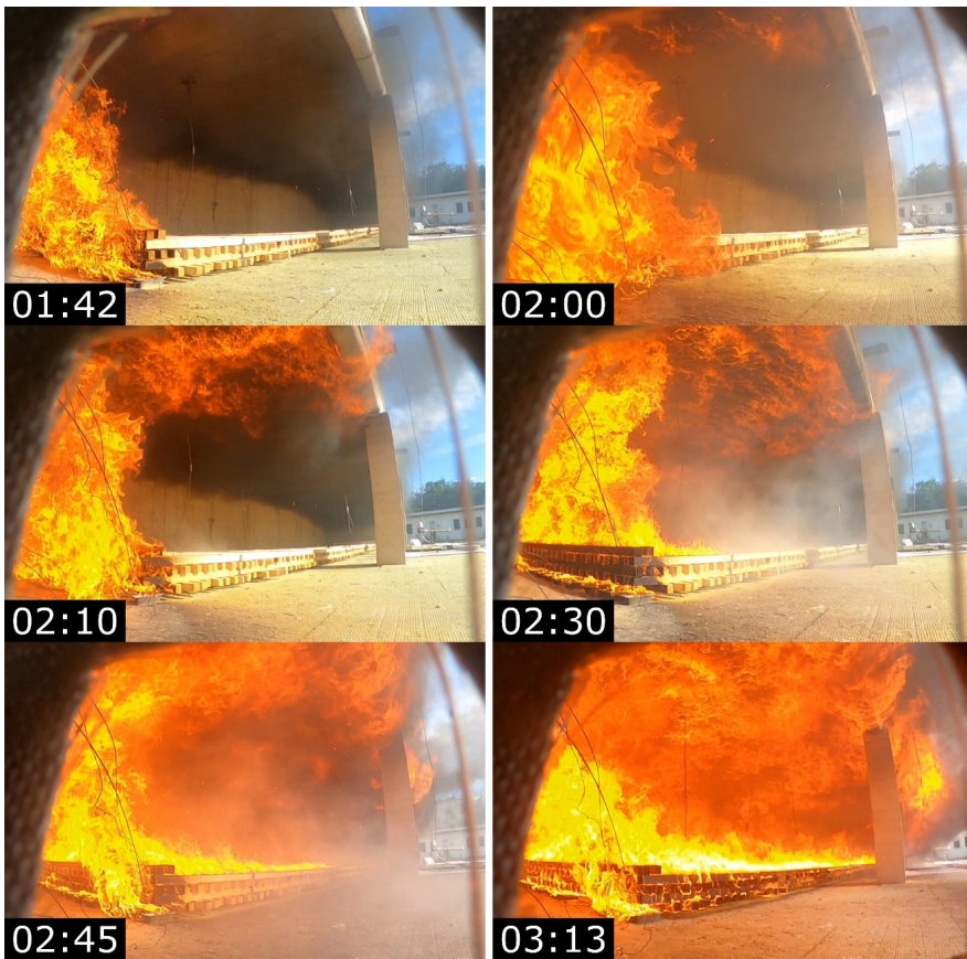
Fig. 17 From ignition of the ceiling, the fire spread across the room in just 91 seconds. Time (mm:ss) after the start of the experiment.
