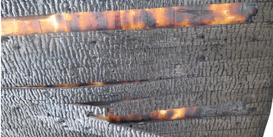
Fig. 15 The image shows partial delamination where several lamellas are partly loose, and some are hanging down. The second layer was mostly discoloured, not charred, which indicates that the temperature at delamination was around 200 °C or lower.
