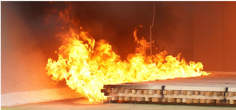
Fig. 53 The heptane fire in #FRIC-01 was tilted away from the wood crib due to local draft conditions, and very little of the wood crib was burning when the heptane fire burned out.
