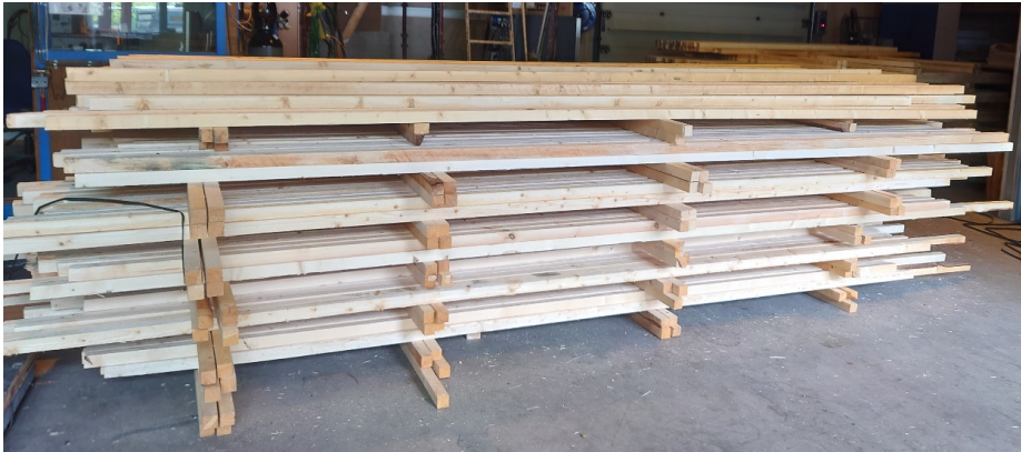
Fig. 52 The wood sticks for the cribs were dried indoors for several months before the experiments.
