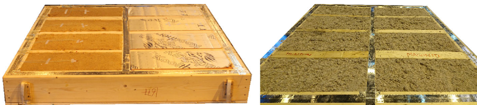
Figure 4. Left: Test specimen filled with wood fibre batt on the left half side and phenolic foam batt on the right half side. Right: Test specimen filled with wood fibre loose-fill insulation (manually packed) between the Hunton I-joists (left) and Masonite I-joists (right). The fibreboard is not installed.
