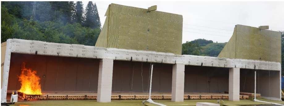
Fig. 3 Photo of the CLT compartment with exposed CLT ceiling. This is of the #FRIC-01 experiment with only the ceiling (not shown) exposed.
