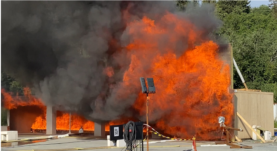
Fig. 22 Image of #FRIC-02 after 3.5 minutes. The external flame covered almost the entire opening of Window 4 directly after flashover, whereas the external flames from the other windows were relatively small.
