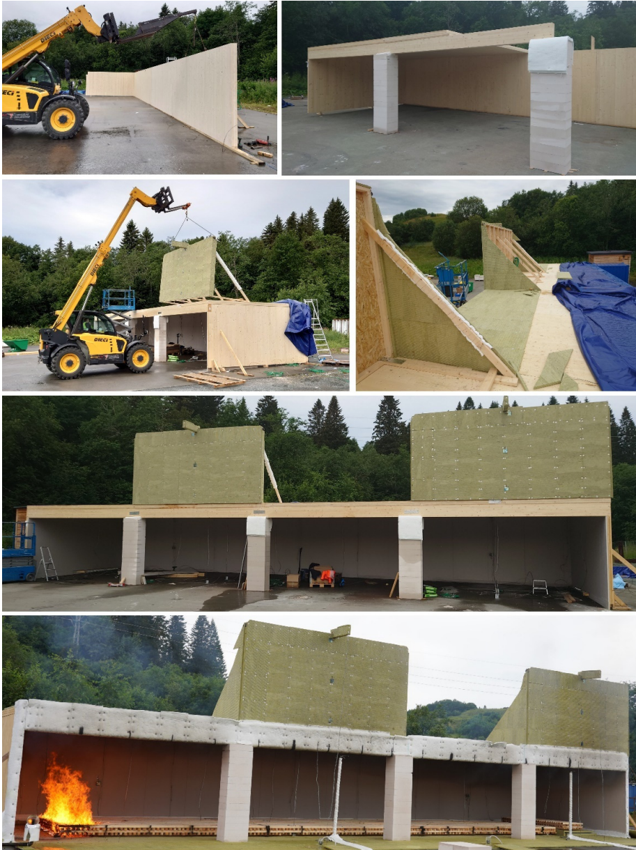
Fig. 46 Images from the rigging of the compartment and the final experimental setup. The image at the bottom is from #FRIC-01.
