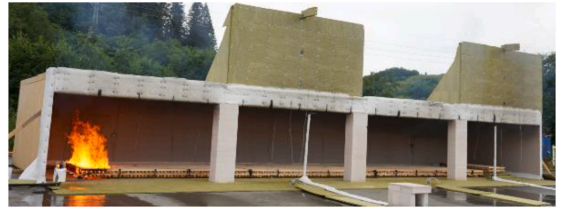
Fig. 2. The compartment with the burning wood crib fire before the ceiling was ignited. The small crib is at the right end of the compartment. The fire shows at which end the wood crib was ignited.
