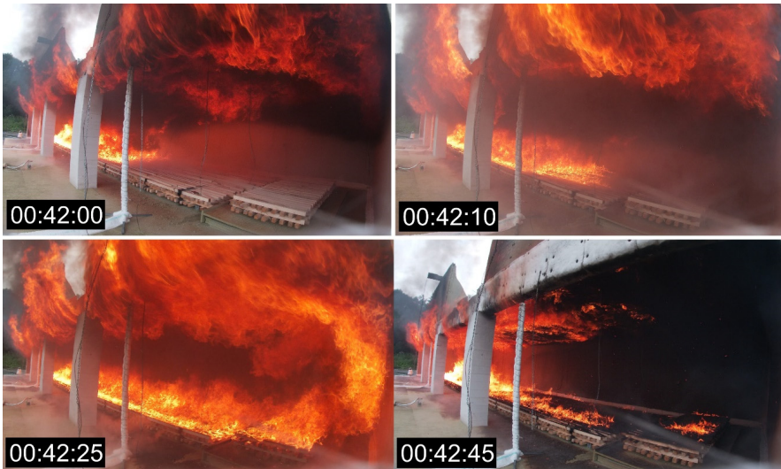
Fig. 7 In the third flashing wave, the fire spread to cover the entire wood crib and ceiling before it retracted shortly after. Time (hh:mm:ss).
