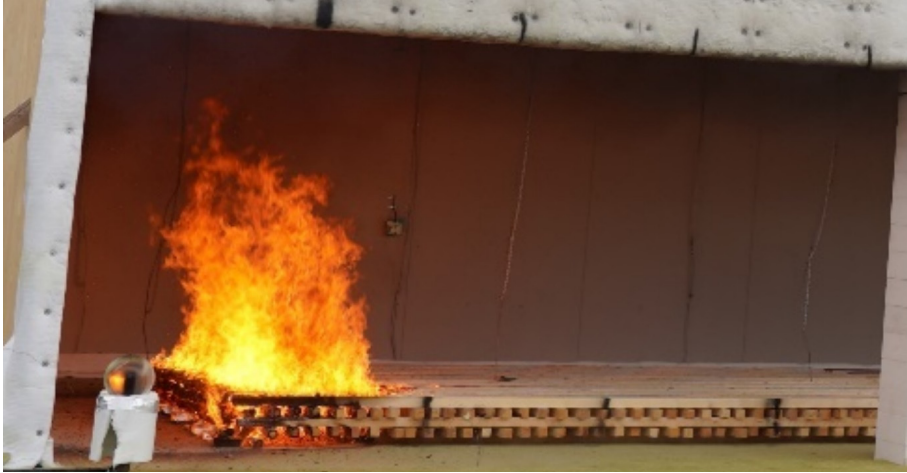
Fig. 5 It took 32.5 minutes before the ceiling was ignited. This image is taken from ca. 20 minutes. This fire spread to 1.5 m before the ceiling was ignited but did not grow larger in size as the first part of the crib was starting to burn out from this point.
