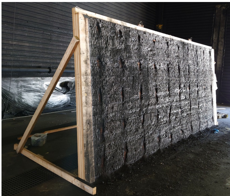
Fig. 68 The elements were raised for easy access from both sides. The vertical stripes are signs of the physically removed char layer around the drilled holes. The element at the picture is one of the ceiling elements from #FRIC-01.
