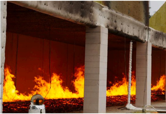
Fig. 13. Cessation of flaming combustion in the ceiling occurred while the wood crib was still burning. Photo from 62 min.
