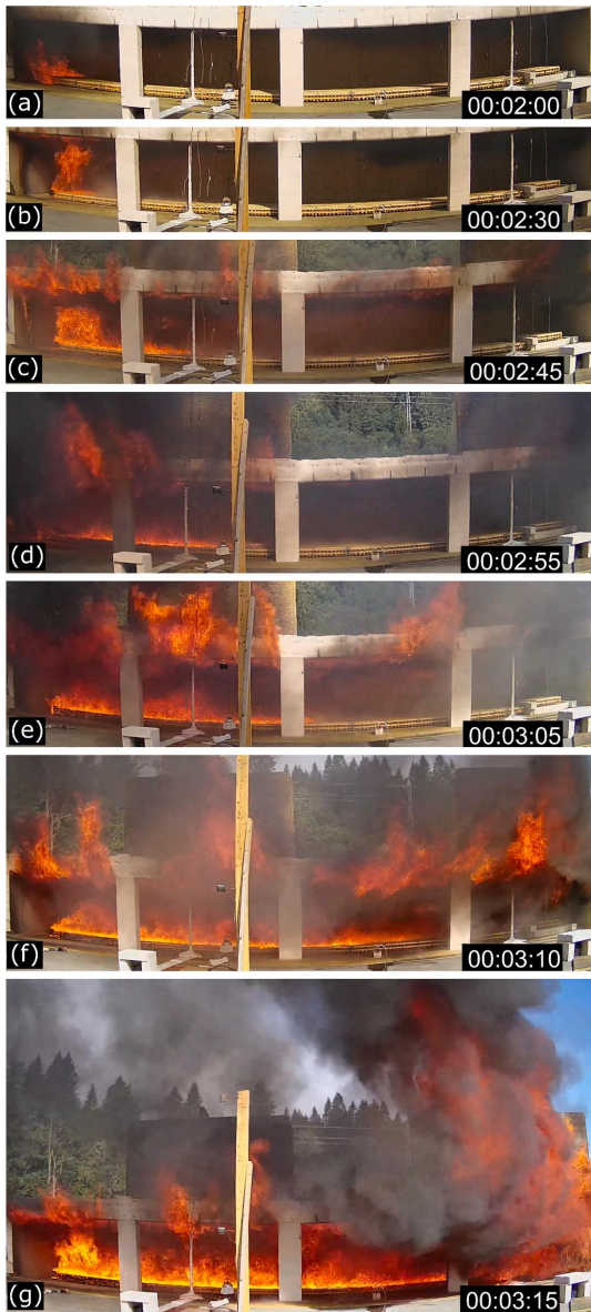
Fig. 7. (a)–(g) Fire spread across the compartment. Time (hh:mm:ss).
