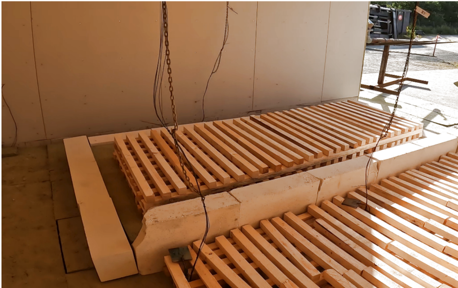
Fig. 55 Image of the small wood crib on the scale. In #FRIC-02, aerated concrete blocks were added to the sides of the scale for better thermal protection.
