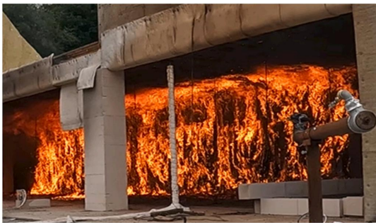
Fig. 11. In the transition to the second flashover, the full height of the back wall was burning before half of the ceiling width had been included in the fire. Photo from 74 min.
