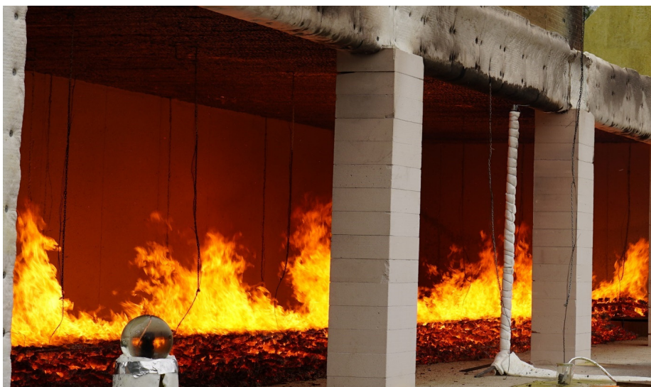
Fig. 14 Self-extinguishment of the flames in the CLT ceiling when the wood crib was still burning.
