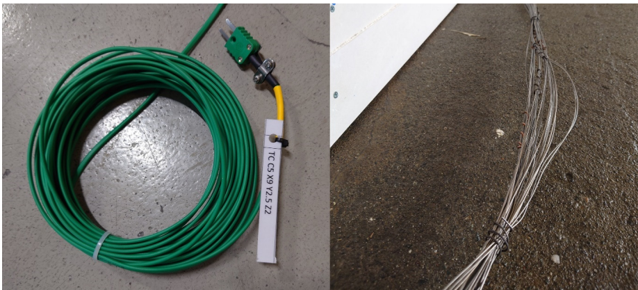
Fig. 61 All sensors were named adequately by a unique ID and organised in bundles.
