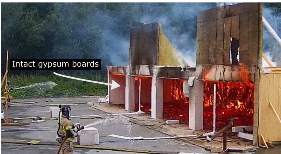
Fig. 44 The gypsum boards at the end walls were intact until the extinguishment of #FRIC-02. The image also shows that the fire was far from being close to self-extinguishing when manually extinguished. Image from 175 minutes
