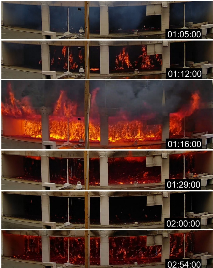
Fig. 20 Development of the second flashover. Time as hh:mm:ss.
