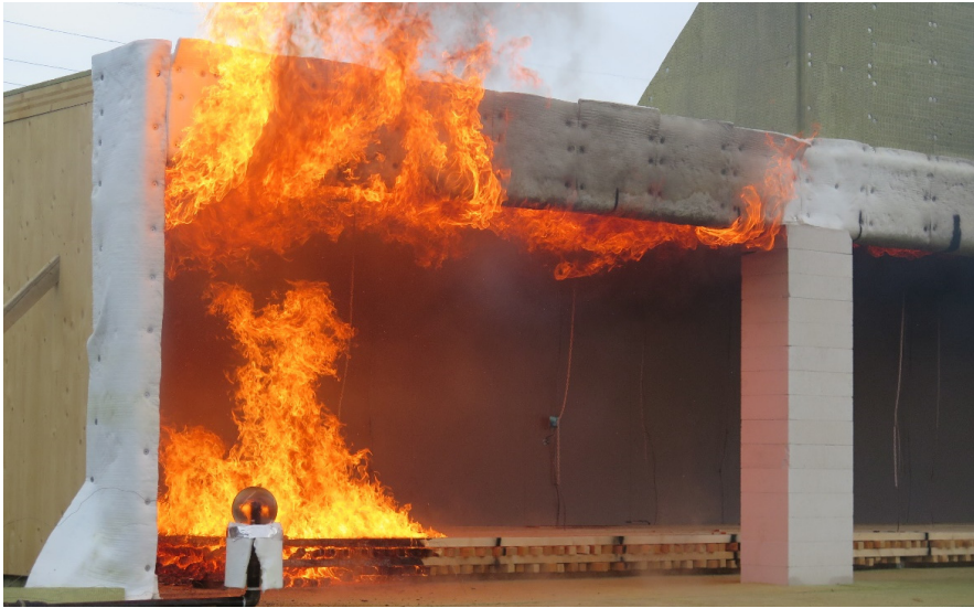
Fig. 6 Flame spread under the ceiling shortly after ignition of the CLT ceiling in #FRIC-01. The image was taken at 33 minutes.
