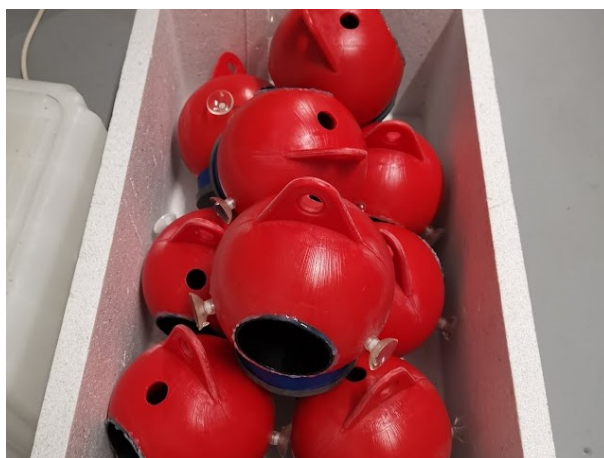
Figure I.2: The underwater camera housing used to connect the cameras to the tank and protect both camera and fish from injuries
