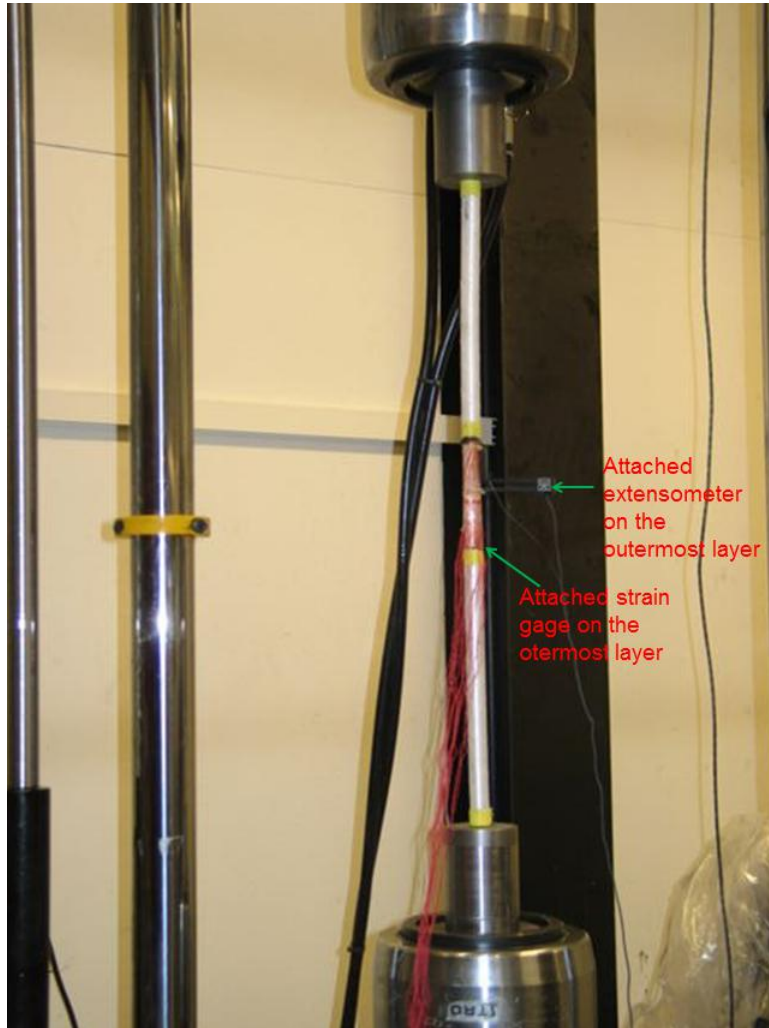
Figure 22: A calibration test for 300 mm^2 copper conductor.
