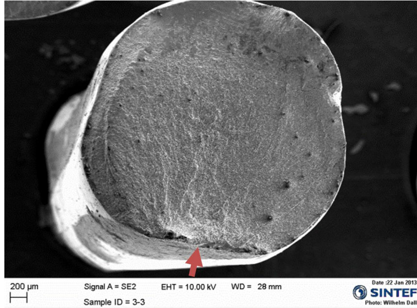
Figure 19: Fracture surface from 3 rd layer of a conductor that had been fatigue tested with radius of curvature \rho_1 = \pm 3000 \text{ mm} .
