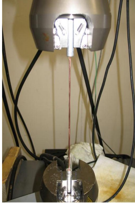
Figure 10: Test rig setup for fatigue test of an individual wire in tension-tension mode with both ends clamped against rotations.
