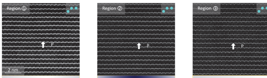
Figure 4-11. HAADF-STEM images from the different regions ①, ②, and ③ of the complex structure showing highly order lattice arrangement. The color bars below each HAADF-STEM image indicate the corresponding conductance states: blue represents enhanced conductance, and white insulates according to the SEM contrast.
