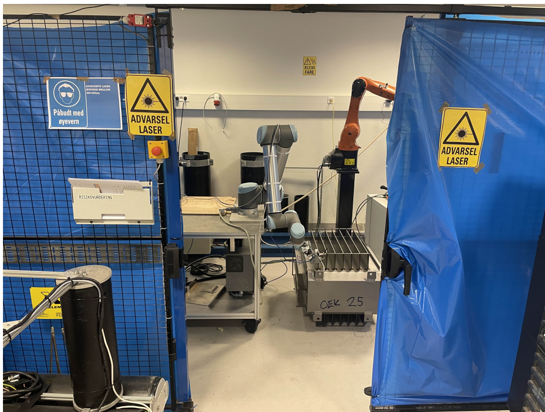
Figure 5.6: Open robot cell with blue plastic tarp. Door can be closed, sealing the cell.
