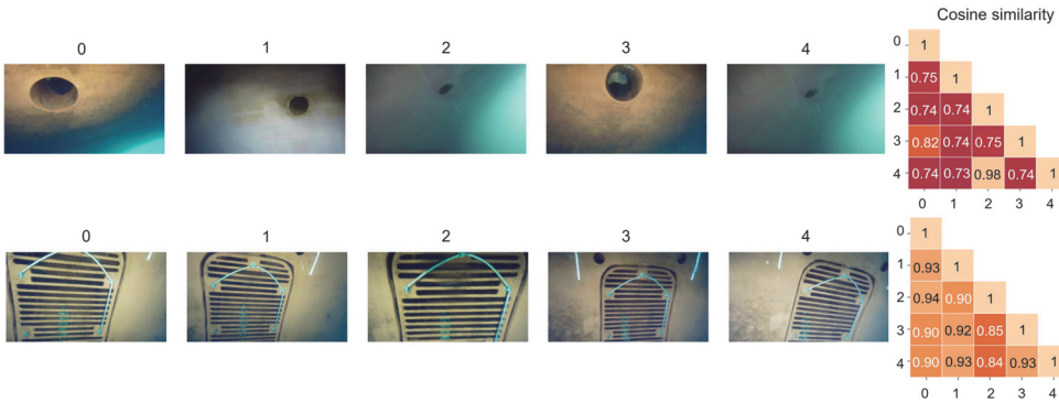
Fig. 7. Similar images of a sea chest grating and an overboard valve with corresponding pairwise Cosine similarity index.
