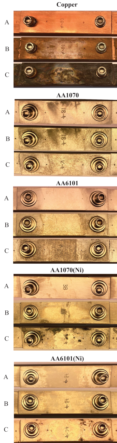
Fig. 6: Photograph of each configuration before corrosion exposure and after B and C level corrosion exposure
