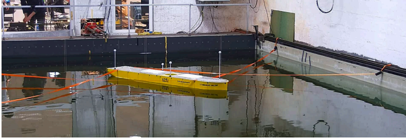
Fig. 9. The model ship C/S Innocean Cat I Drillship (CSAD) used in experiments. The position and orientation were held fixed by ropes with 1 kg weights attached to each end. Image reproduced with courtesy of Udjus (2017).
