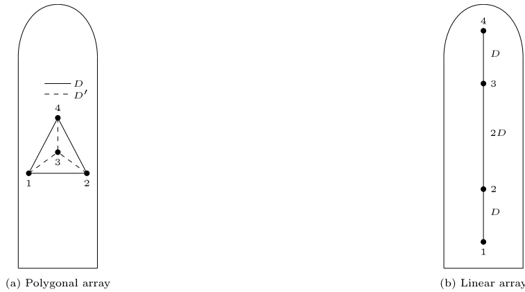
Fig. 4. An illustration of the different sensor arrays considered in the analysis of Section 4. The sensors {1,2,4} in (a) form an equilateral triangle on the horizontal plane with length D and a circumscribed circle at {3} with radius D' = D/\sqrt{3} .
