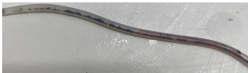
Figure 2.36: A photograph of a fouled tube using Fomblin as a carrier fluid. The black materials are wetted aggregated quantum dots due to long usage.
