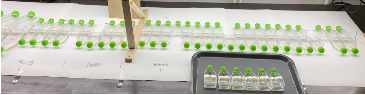
Figure D. 3: A photo showing the experimental setup of the experiment testing addition of nutrients. The photo shows the cell cultivation flasks, laying horizontally on a white cover board below the light source. The picture also illustrate how cell cultivation flasks were transported to the inverse microscope for investigation.
