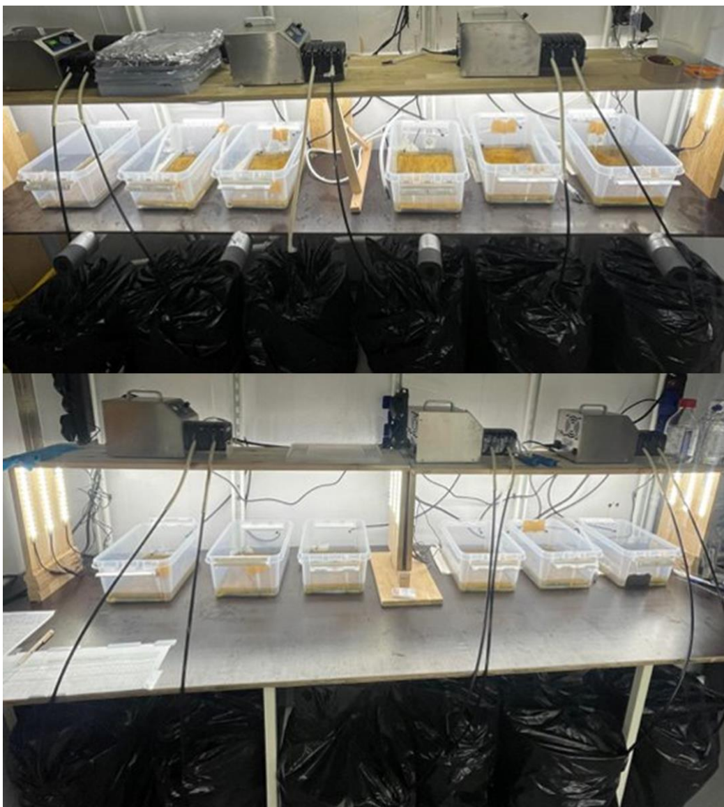
Figure D. 4: A photo showing the experimental setup of the experiment testing harvest rate. At the top, reactor 1-6, with respective water supply beneath the light bench. The peristaltic pumps are placed above the light bench. At the bottom, reactor 7-12, with the same setup as for reactor 1-6. The water cans (50L) were covered in black plastic bags (seen beneath the reactors) to ensure no photoautotrophic growth in the cans.
