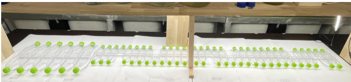
Figure D. 2: A photo showing the experimental setup of the experiment testing addition of Silica. The photo shows the cell cultivation flasks, laying horizontally on a white cover board below the light source. The three empty spots illustrate how the cell cultivation flasks were picked for investigation in the inverse microscope.
